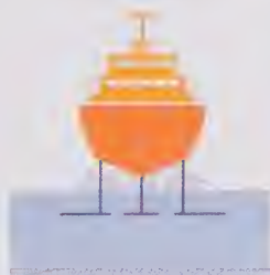
FULLY SUBMERGED HYDROFOIL
